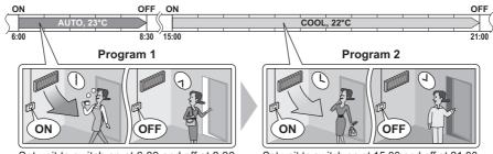
Set unit to switch on at 6:00 and off at 8:30 Chosen mode: Auto/Set temperature: 23°C Set unit to switch on at 15:00 and off at 21:00 Chosen mode: Cool/Set temperature: 22°C
