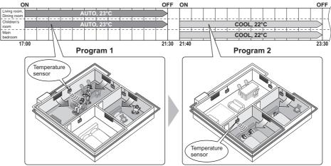
Set unit to switch on at 17:00 and off at 21:30 Chosen mode: Auto/Set temperature: 23°C Chosen zone: Living, Dinning, Children room Chosen temperature sensor: Living room Set unit to switch on at 21:40 and off at 23:30 Chosen mode: Cool/Set temperature: 22°C Chosen zone : Main bedroom, Children room Chosen temperature sensor: Main bedroom
